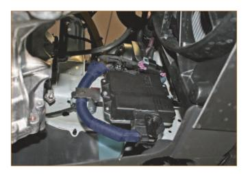
Pict. 16 ECU assembly into the engine compartment
