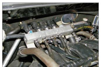
Pict. 4 Example of installation of Rail with BRC injectors and gas pressure and temperature sensor
