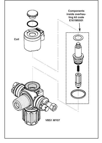
Remove wrinkled pipes, unscrew steel pipes and unhook Coil connector. Disassemble cylinder, unhooking it form its support. Fix cylinder in order to unscrew VBS1 MY07. Use a 27 mm wrench or a 1/2" 🖄 ratchet spanner. Clean and check thread. Using a new VBS1 MY07, follow the
