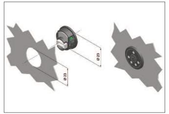
Pict. 17 One-Touch changeover switch example of built-in fixing
