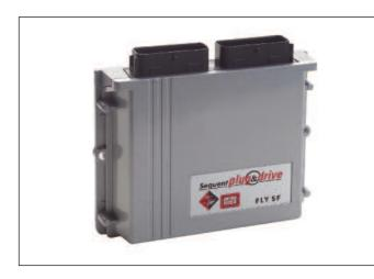
ber that ECU has been planned to withstand prolonged short-circuits, both towards ground and battery positive, on each of its inlet/outlet cables (naturally except for grounds and supplies). This allows not ruining ECU even in presence of the most common wiring errors (polarity inversion, wrong connection of one or more cables, etc.).
