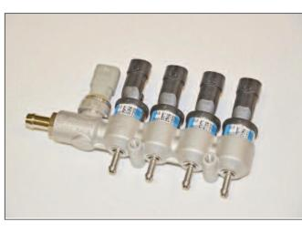
Pict. 4a Version with BRC MY09, injectors, gas pressure and temperature sensor
