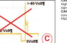
CASE C High voltage coi signal. Vehicle CAN NOT be converted with P&D SCORPIO
