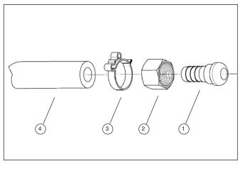
Pict. 7 Assembly of pipe-holder on pipe
