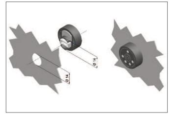
Pict. 18 One-Touch changeover switch example of external fixing
